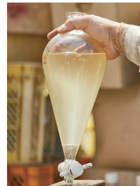
The distilled liquid separates into essential oil and herb water after being left for some time. Let the herb water flow down from the bottom, leaving only the essential oil.
