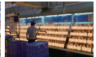
The assembled aroma diffuser goes through a process called ageing, which runs a three hours long testing, where the final product is completed and sent to MUJI all over the world.
